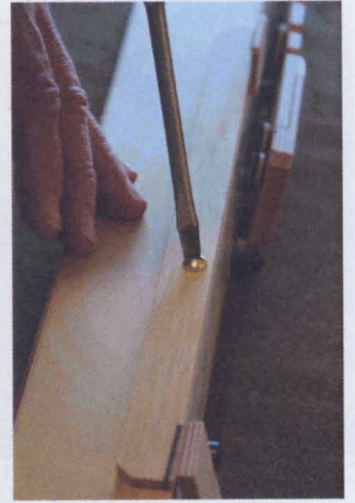
Image 12: Loosening the key levers
