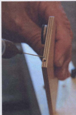
Image 18: Oiling the axle guides
